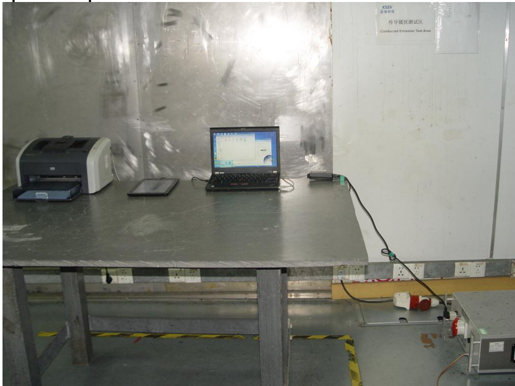
Photograph 2: Set-up for Radiated Emission of below 1GHz
