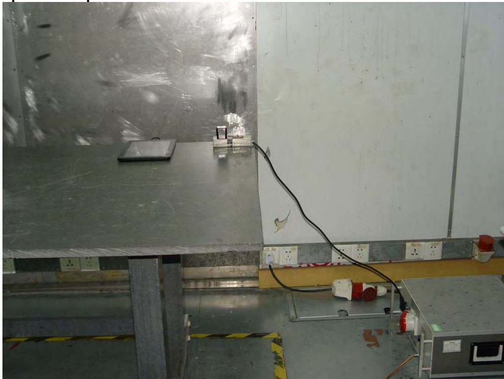
Photograph 1: Set-up for Conducted Emission
