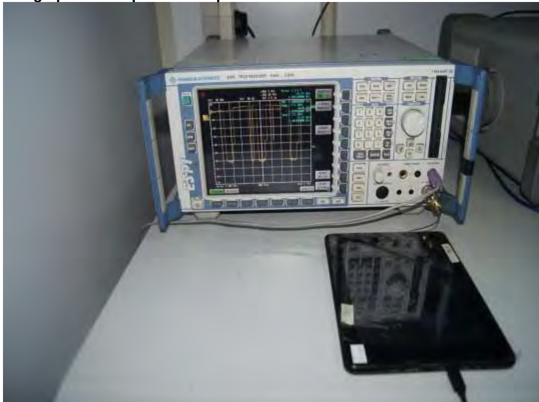
Photograph 6: Set-up for radio spectrum test
