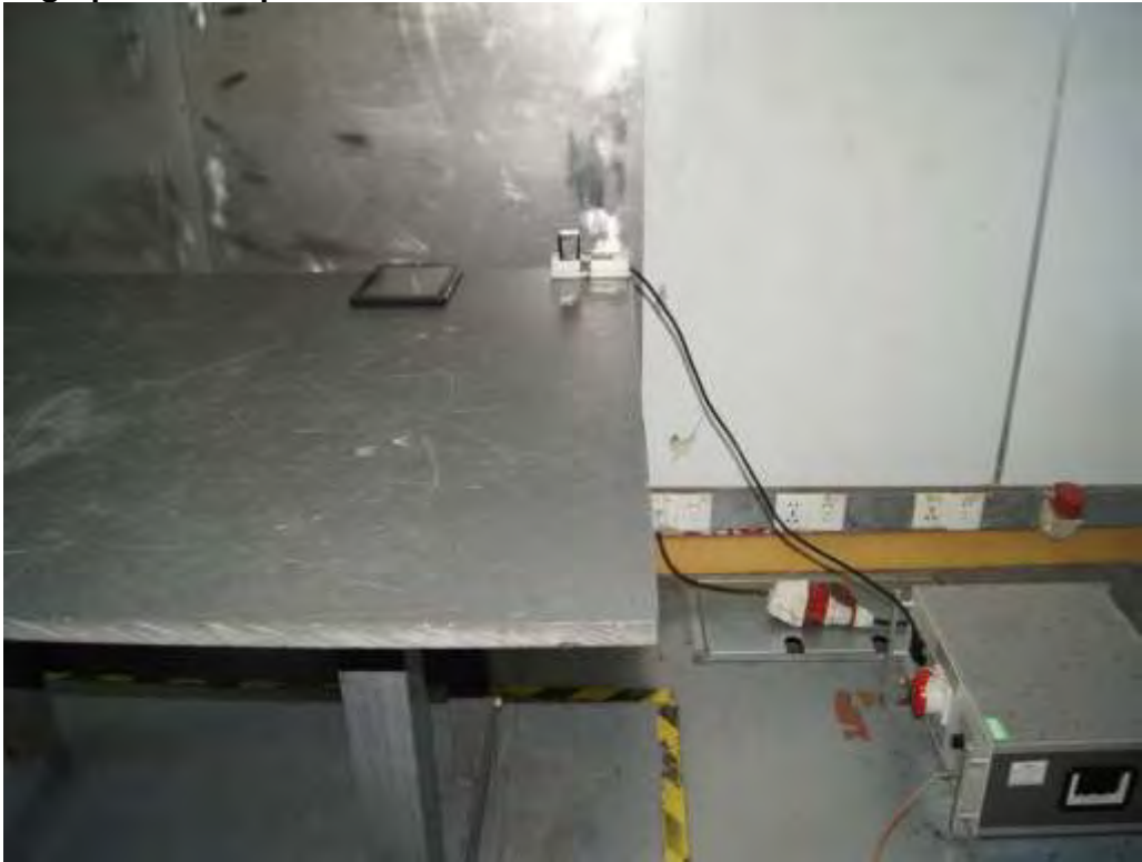
Photograph 2: Set-up for Spurious Emissions below 30MHz
