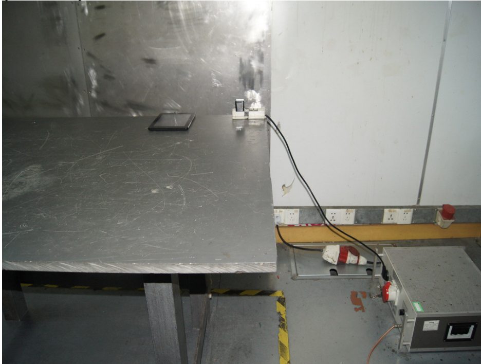
Photograph 2: Set-up for Radiated Emission of below 1GHz
