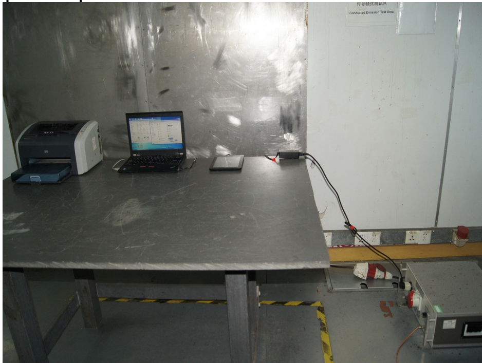
Photograph 2: Set-up for Radiated Emission of below 1GHz
