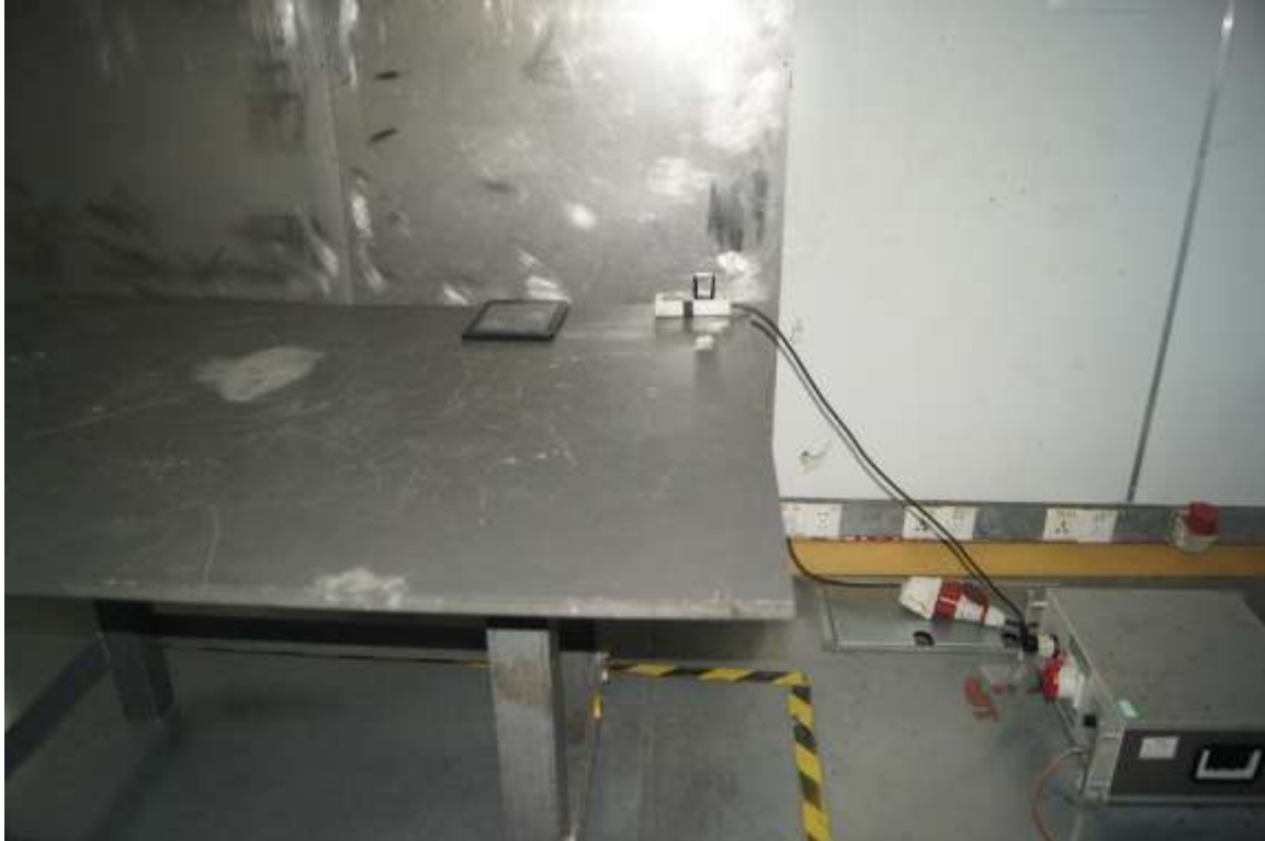
Photograph 2: Set-up for Spurious Emissions below 1GHz
