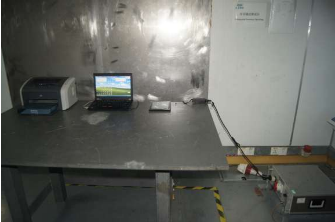
Photograph 2: Set-up for Radiated Emission
