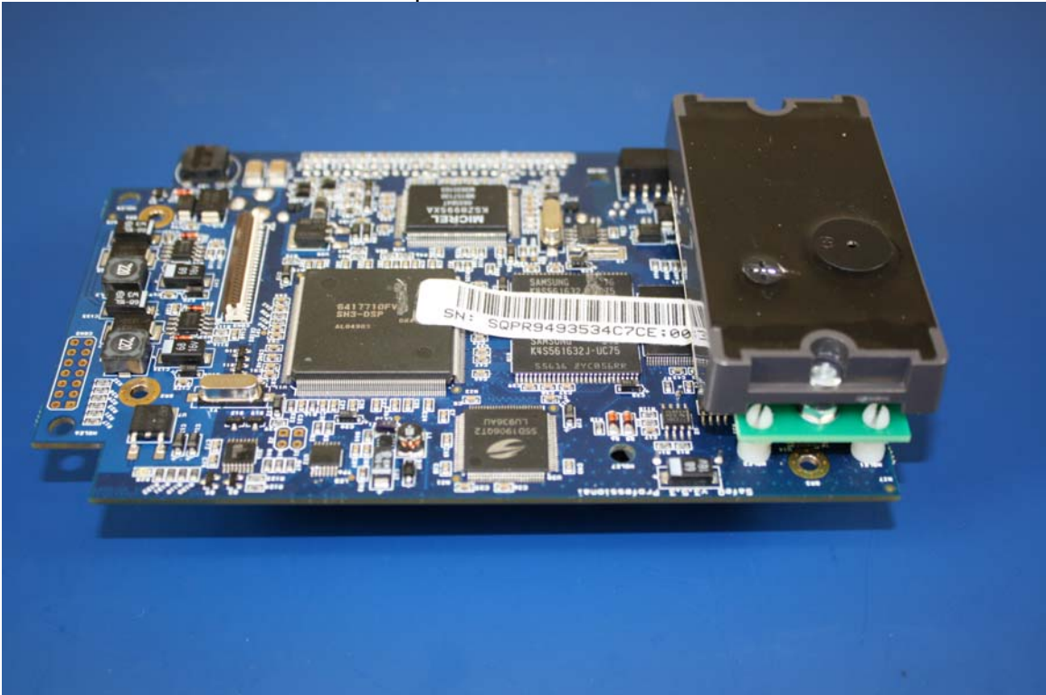
Internal – Top View - Board Stack with radio
