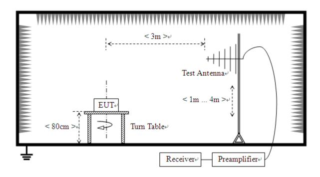
The test is performed in a 3m Semi-Anechoic Chamber; the antenna factor, cable loss and so on of the site (factors) is calculated to correct the reading. The EUT is placed on a 0.8m high insulating Turn Table, and keeps 3m away from the Test Antenna, which is mounted onavariable-height antenna master tower.
