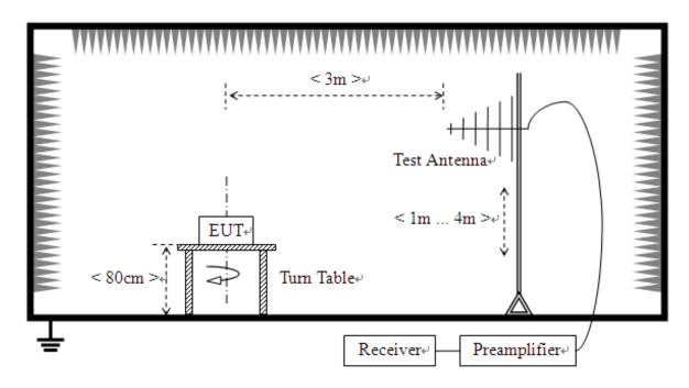
The test is performed in a 3m Semi-Anechoic Chamber; the antenna factor, cable loss and so on of the site (factors) is calculated to correct the reading. The EUT is placed on a 0.8m high insulating Turn Table, and keeps 3m away from the Test Antenna, which is mounted onavariable-height antenna master tower.
