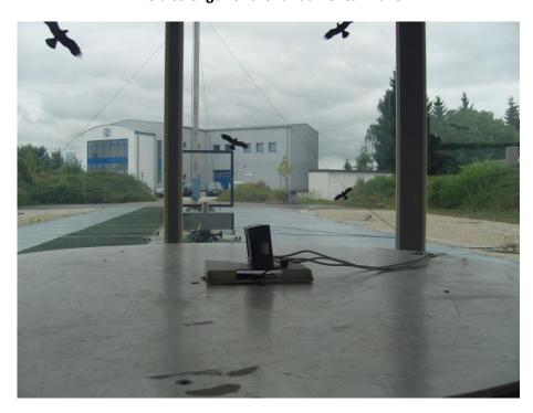
Spurious emissions (magnetic field) 9 kHz - 30 MHz
