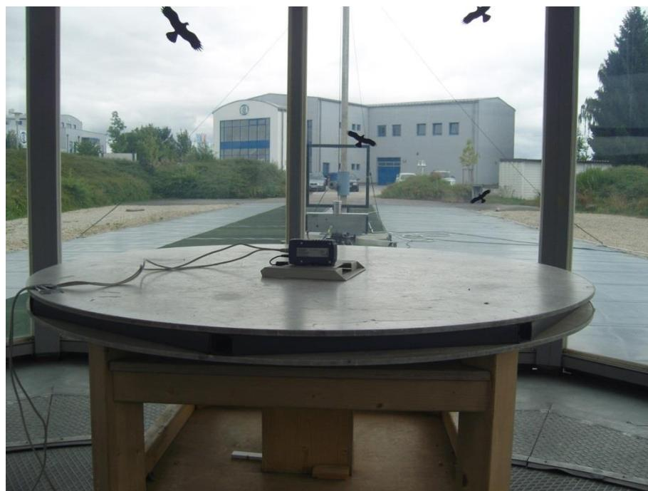
**Spurious emissions (magnetic field) 9 kHz – 30 MHz**
