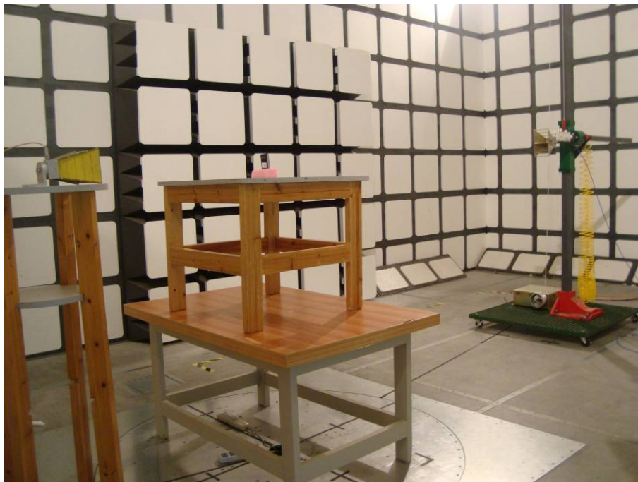
Above 1GHz: Spurious Radiated Emissions - Rear View
