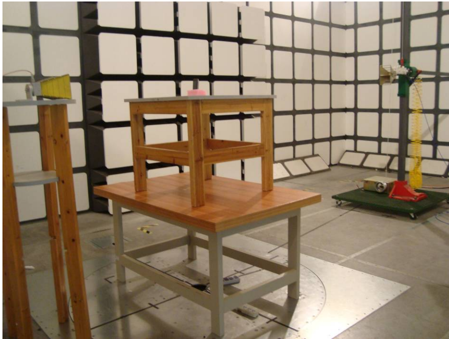
Above 1GHz: Spurious Radiated Emissions - Front View
