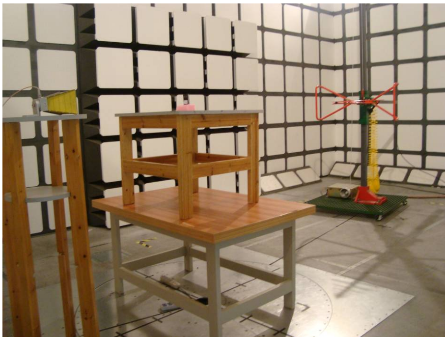
Below 1GHz: Spurious Radiated Emissions - Rear View
