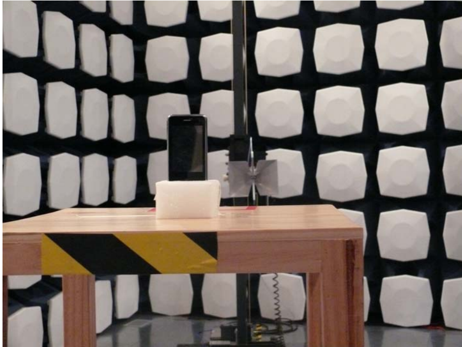
Picture 2: Radiated Spurious Emissions Test setup
