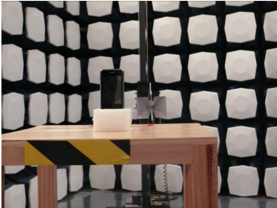
Picture 2: Radiated Spurious Emissions Test setup
