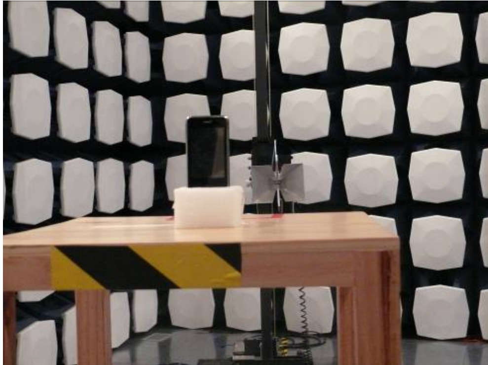
Picture 2: Radiated Spurious Emissions Test setup
