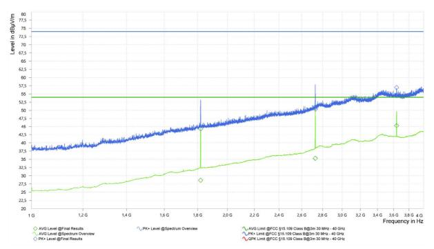
Spurious emissions from 1 GHz to 4 GHz (normal operation mode 1):
