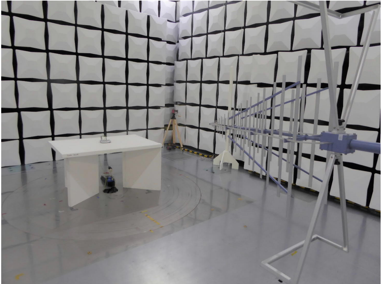
Test setup semi anechoic chamber
