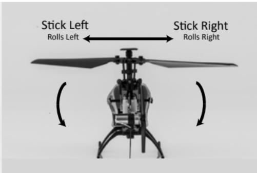
Moving the right-hand stick to the left will roll the helicopter to the left, allowing it to be flown to the left. Moving the right-hand stick to the right will roll the helicopter to the right, allowing it to be flown to the right.
