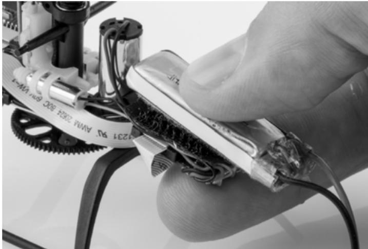
First turn on the transmitter and then plug the battery into the 4-in-1 controller being careful to maintain correct polarity
