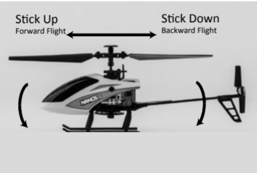
The right-hand stick controls both the elevator (pitch fore/aft) and aileron (roll) channels. Pushing the stick forward will pitch the nose of the helicopter downward, allowing it to be flown forward. Pulling the stick down pitches the nose of the helicopter upward, allowing it to be flown backwards.
