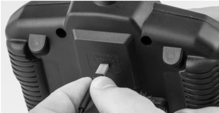
To charge the flight battery, plug the included charge cord into the rear of the transmitter. Plug the battery into the other end of the charge cord. The LED on the front of the transmitter will light green when charging and go out when the battery is charged.
