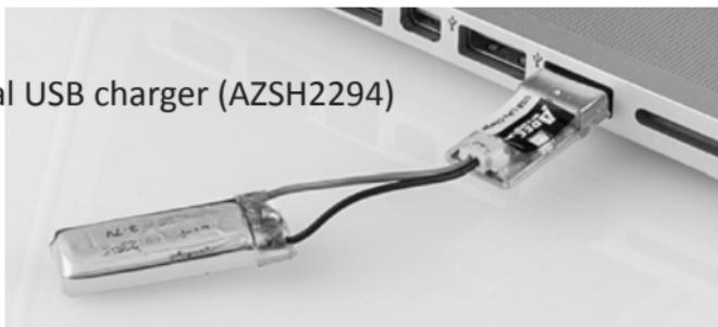
To charge the flight battery using the optional USB charger (AZSH2294) plug battery into USB charger and plug charger into USB port on computer. Red LED indicates charging, Green LED lights when battery is charged.
