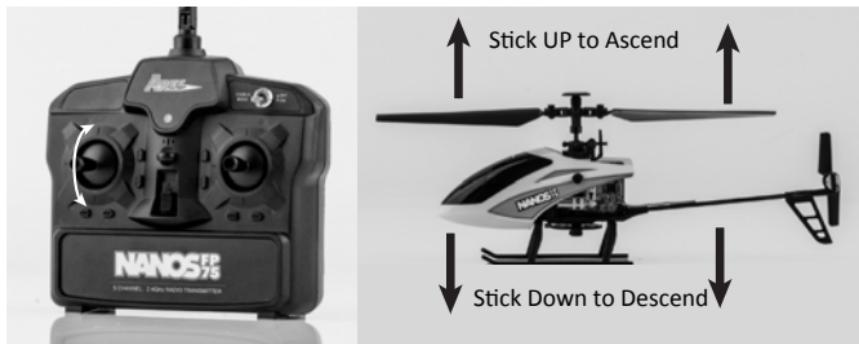
The left-hand stick on the transmitter controls both the throttle (climb/descend) and rudder (yaw left/right) channels. Moving the stick up increases the speed/RPM of the rotor blades and causes the helicopter to climb. Lowering the stick reduces the speed/RPM and causes the model to descend.
