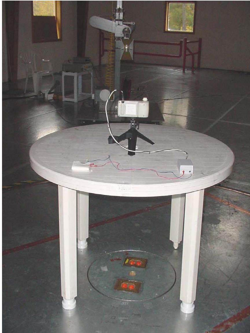
Radiated Emissions above a 1GHz – Rear View
