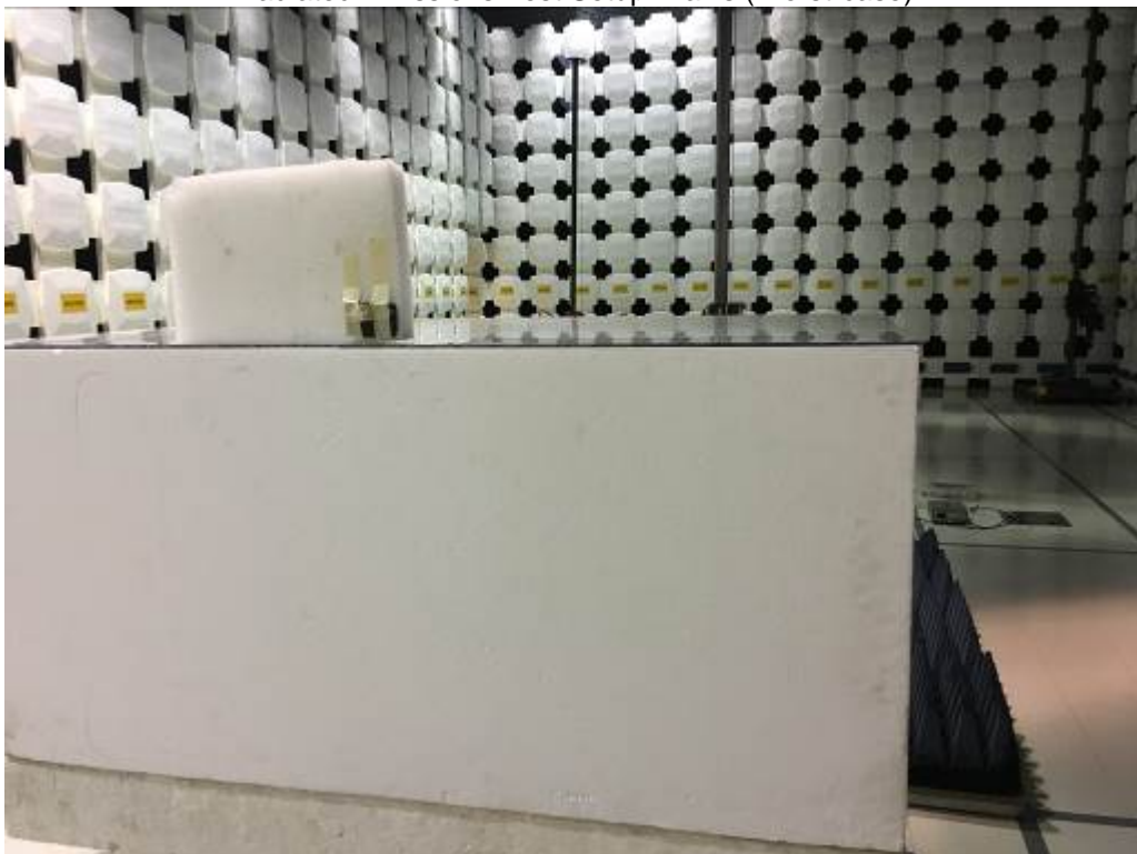
Radiated Emissions Test Setup Y-axis (Worst-case)
