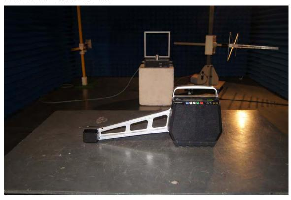
Radiated emissions test 30MHz-1GHz
