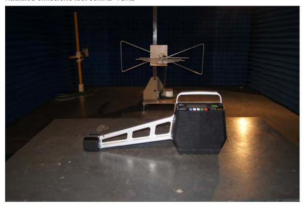
Radiated emissions test > 1GHz
