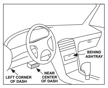
2. For most vehicles, use OBD2 Diagnostic Cable to connect DLC and WSM. Power indicator will light up on WSM when connected.
