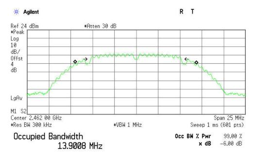
Transmit Freq Error -60.297 kHz x dB Bandwidth 10.359 MHz
