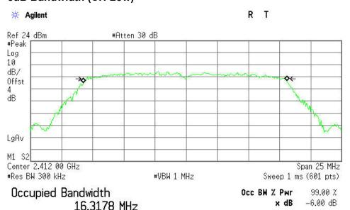
Transmit Freq Error -72.064 kHz x dB Bandwidth 15.946 MHz
