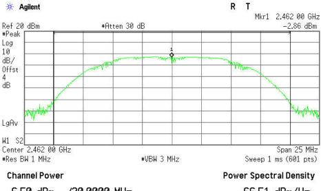
6.50 dBm /20.0000 MHz -66.51 dBm/Hz
