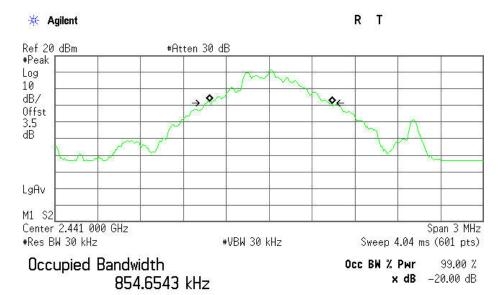
Transmit Freq Error 10.473 kHz x dB Bandwidth 854.805 kHz
