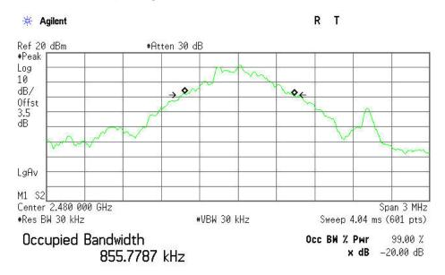
Transmit Freq Error 12.802 kHz x dB Bandwidth 861.399 kHz
