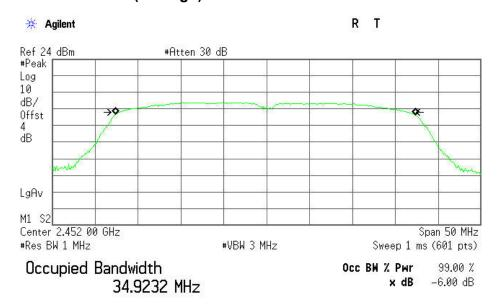
Transmit Freq Error -113.463 kHz x dB Bandwidth 33.779 MHz
