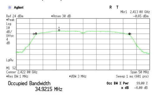
Transmit Freq Error -119.747 kHz x dB Bandwidth 33.799 MHz
