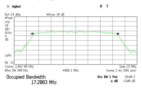
Transmit Freq Error -46.046 kHz x dB Bandwidth 16.434 MHz
