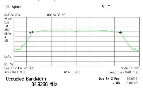
Transmit Freq Error -124.958 kHz x dB Bandwidth 33.615 MHz
