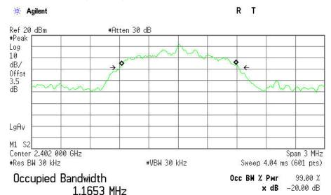
Transmit Freq Error 8.956 kHz x dB Bandwidth 1.212 MHz
