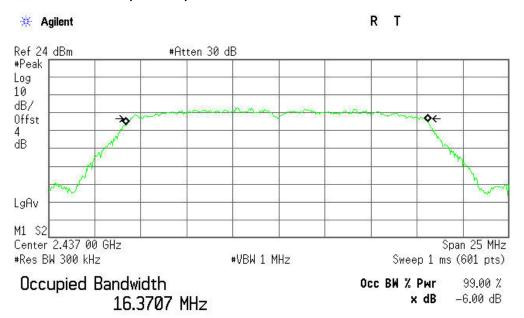
Transmit Freq Error -94.001 kHz x dB Bandwidth 15.912 MHz
