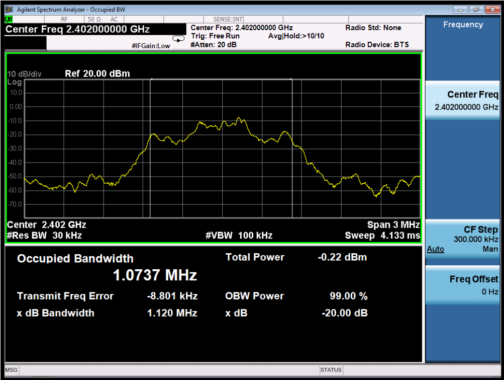
TEST PLOT OF BANDWIDTH FOR LOW CHANNEL
