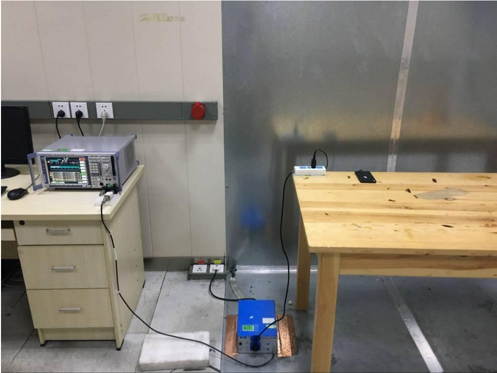
FCC RADIATED EMISSION TEST SETUP BELOW 1GHZ
