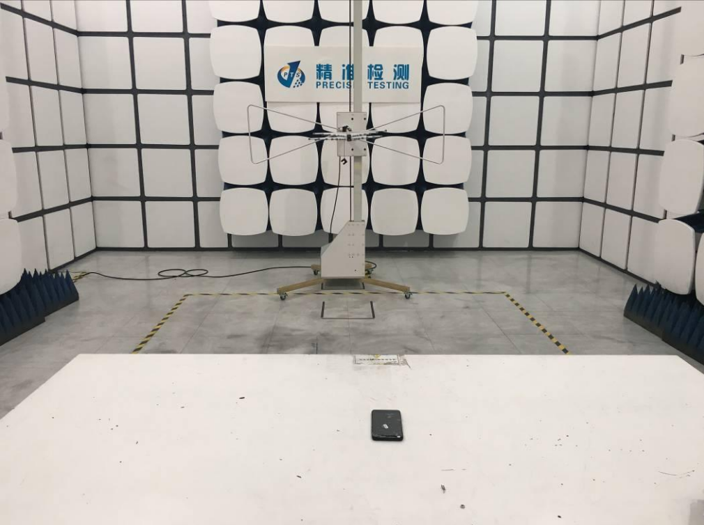
FCC RADIATED EMISSION TEST SETUP BELOW 1GHZ
