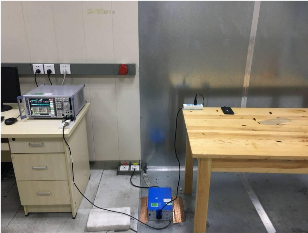
FCC RADIATED EMISSION TEST SETUP BELOW 1GHZ
