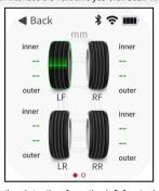
3. The system starts the detection from the left front wheel of the vehicle by default, but you can also manually select any tire for detection. After clicking on the tire icon, attach the magnetic head of the device to the tread of the corresponding tire, and press the measurement button on the device to start the detection. At this time, a scanning animation is displayed on the
