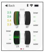
After all tire tests are completed in turn, the tire icon will identify the tire detection results in different colors.
