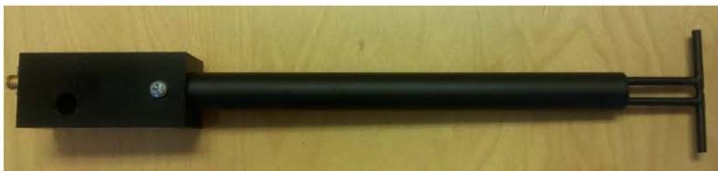
Figure 1 – MVG COMOSAR Validation Dipole
