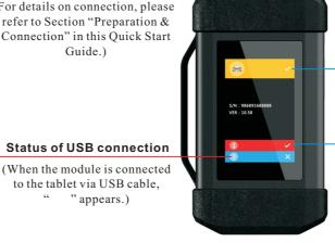
The HD IV module works as a vehicle communication interface device, which is designed to read the vehicle data and then send it to X-431 PAD IV tablet via Bluetooth communication and USB connection. The module comes loaded with a 4" display screen, enabling you to easily identify the working status of the module and X-431 PAD IV tablet.
