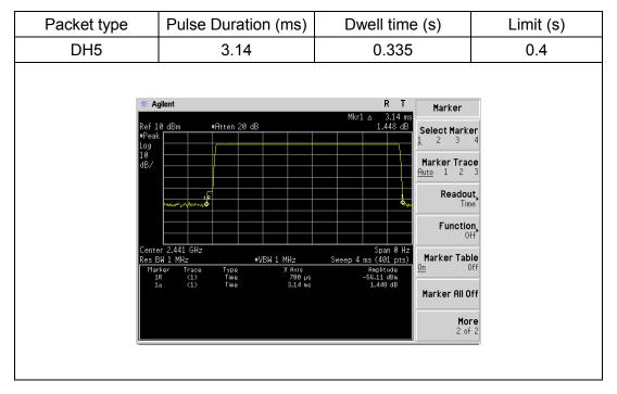
Note: for the worst mode of DH5 packet type, in normal hopping mode, hopping rate is 1600hops/s with 6 slots in 79 hopping channel
