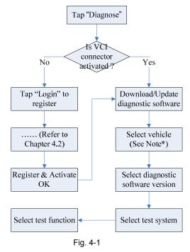
\*Note: If "VIN Scan" or "Intelligent Diagnosis" is selected to diagnose a vehicle, this step shall not apply.
