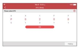
Swipe the screen upwards/downwards to alter the value, then press [OK] button, the screen will display definition of the DTC.
