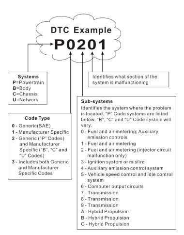
P0201 - Injector circuit malfunction, Cylinder 1
