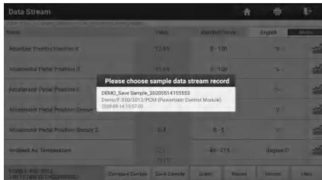
All the values you customized and saved in process of DS sampling will be imported into the **Standard Range** (See below) column for your comparison.
