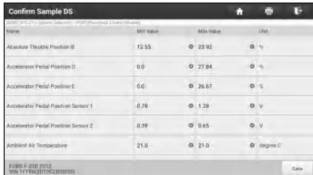
The screenshot shows a 'Confirm Sample DS' interface with a table of data stream parameters. The table has columns for Name, Min Value, Max Value, and Unit. A 'Save' button is at the bottom right.
