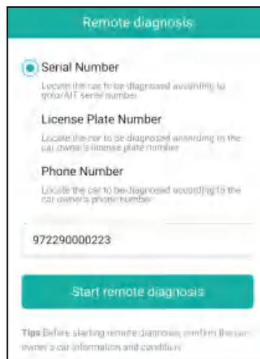
4. Tell the partner to check the box **Serial number** and enter the Serial Number provided by you, and then tap **Start remote diagnosis** to control your device remotely.
