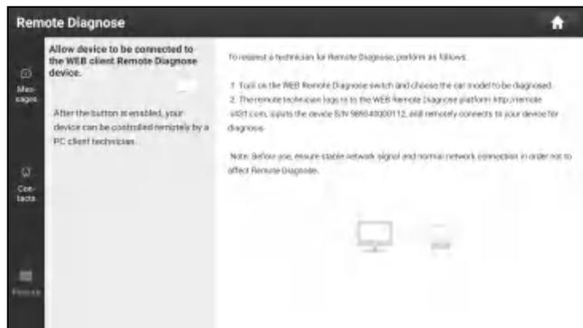
1. Slide the switch **Allow device to be connected to the WEB client remote diagnostic device** to ON so that the partner can find and connect to this device while using the PC.
