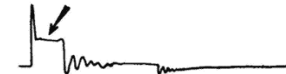
Spark plug gap is too large or mixture gas is too lean
