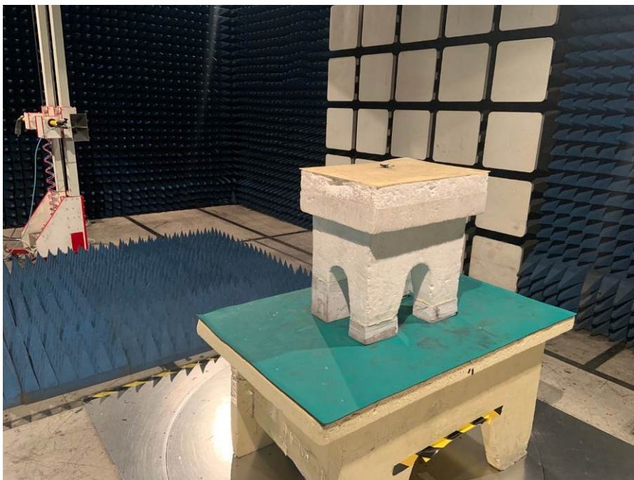
Spurious Emission Test Setup (Above 1GHz)
