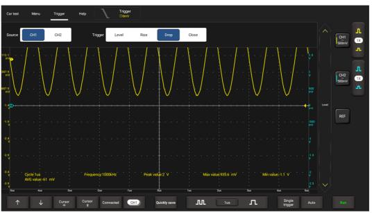
The EM101N applies edge trigger, which is the most commonly used and effective trigger method. A clear majority of applications apply this trigger method to trigger waveform. An edge trigger determines whether the Oscilloscope finds the trigger point on the rising/falling/dual edge of a signal. When the
