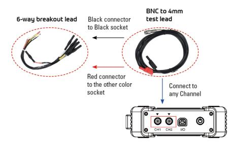
2. Connect the black terminal and signal wire (its other end connected to the red 4mm connector) of the 6-way breakout lead to the GND and signal terminal of the vehicle sensor.
