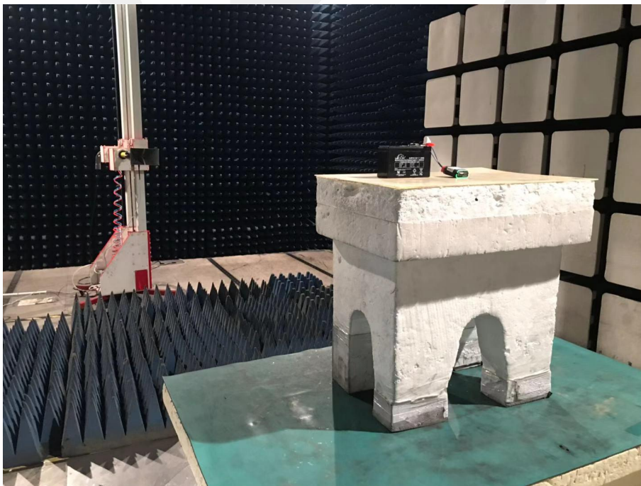
Spurious Emission Test Setup (Above 1GHz)
