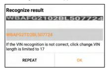
If the VIN scanned is incorrect, tap the result field to modify it and then tap **OK**. If the VIN exists on the remote server, the system will navigate to the diagnostic function selection screen directly.
