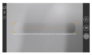
Place the VIN inside the viewfinder rectangle to scan it. The most recognizable location for this number is in the top left corner on the vehicle's dashboard. Other locations include the driver's door or post, and the firewall under the hood.
