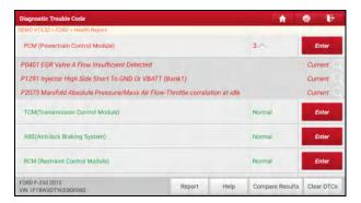
The tested system with fault code appears in red and the system functioning properly displays in black (normally).
