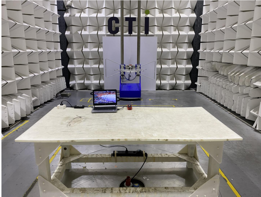
Radiated spurious emission Test Setup-1(Below 1GHz)
