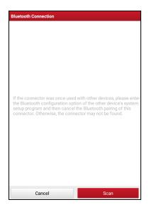
Tap "Scan" to start searching for the VCI. Once it is found, tap it to start pairing. If the tablet has paired with the VCI, it will enter Step 2 directly.
