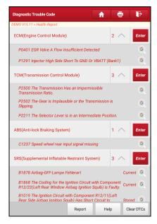
The tested system with fault code appears in red and the system with OK displays in black (normally).
