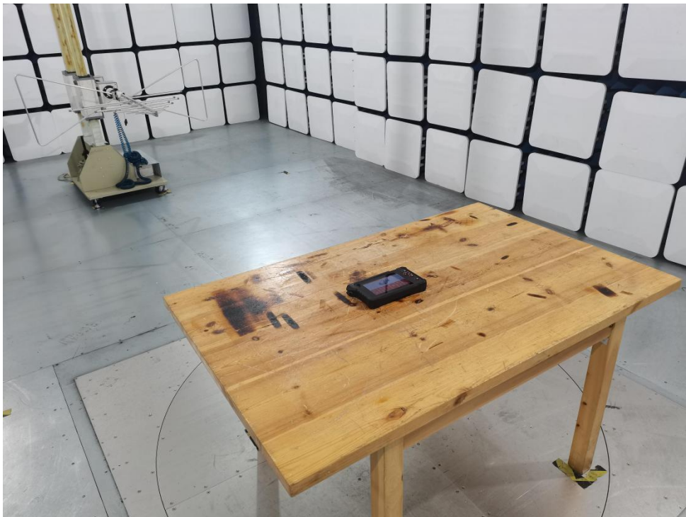
Photo of Radiation Emission Test
