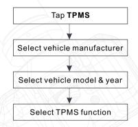
Note: For indirect TPMS vehicle, only the Relearning function is supported.
