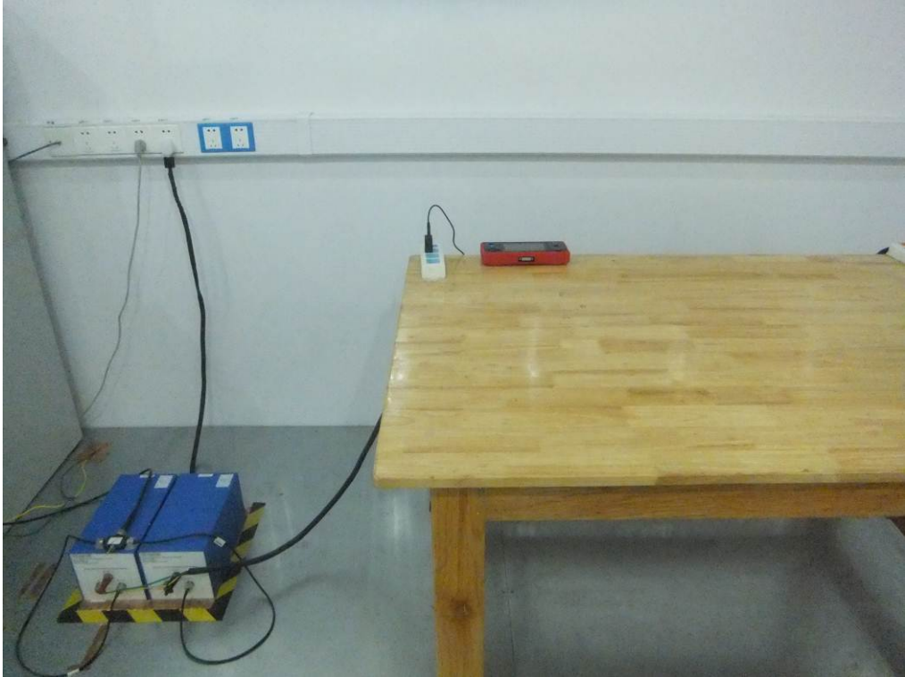
Conducted Emissions Test Setup Front View
