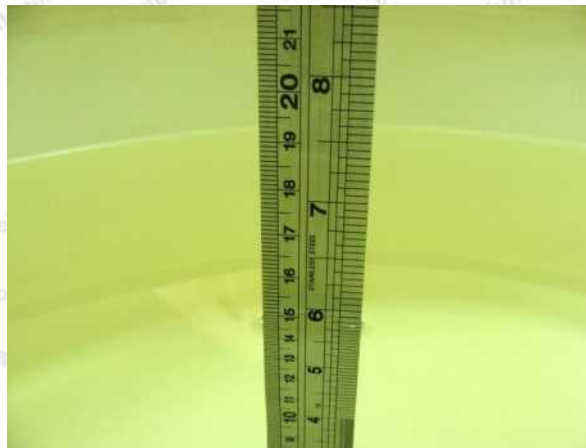
Photo of Liquid Height for Body SAR
