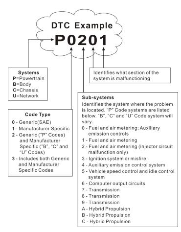
P0201 - Injector circuit malfunction, Cylinder 1
