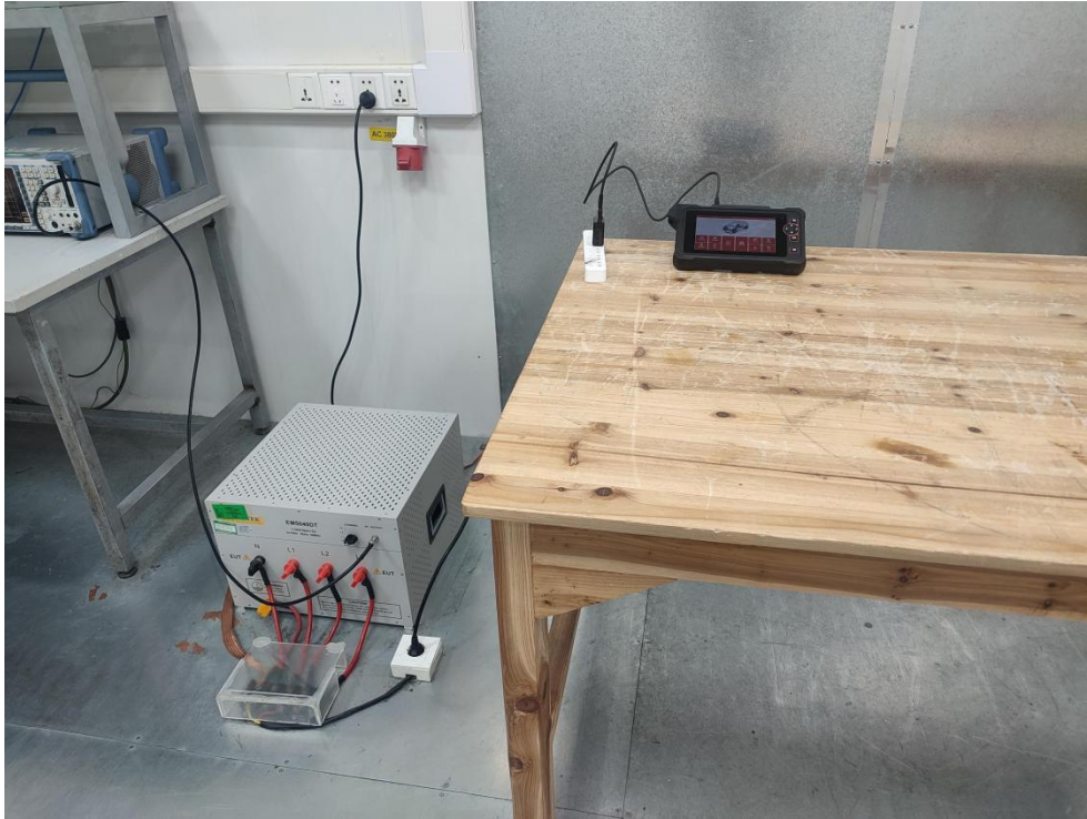
Photo of Power Line Conducted Emission Test
