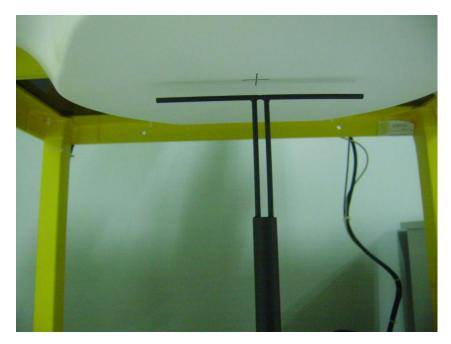
**Setup Photo of Dipole Antenna**
