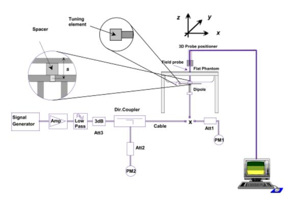
**System Verification Setup Block Diagram**
