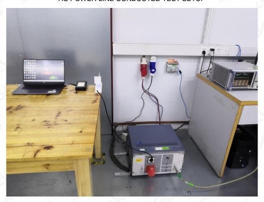
RF CONDUCTED TEST SETUP
