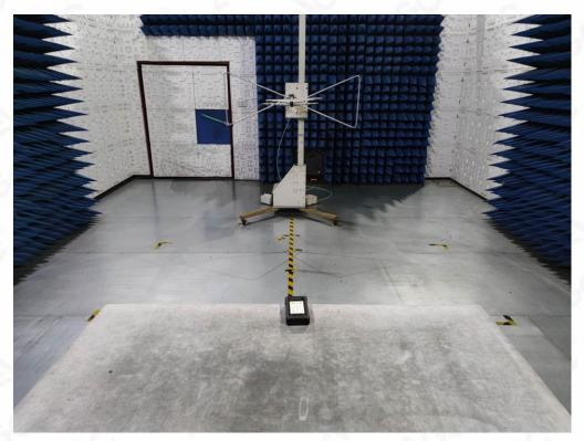
RADIATED EMISSION TEST SETUP ABOVE 1GHz
