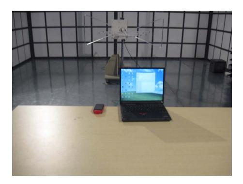
Radiation Emission Test Setup (Above 1GHz)
