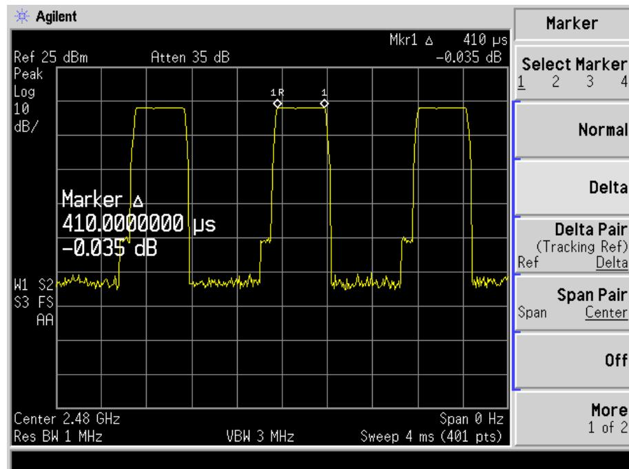
$$\text{DH1 time slot} = 0.41 (\text{ms}) * (1600/(79)) * 31.6 = 262.4 (\text{ms}) < 400 (\text{ms})$$
