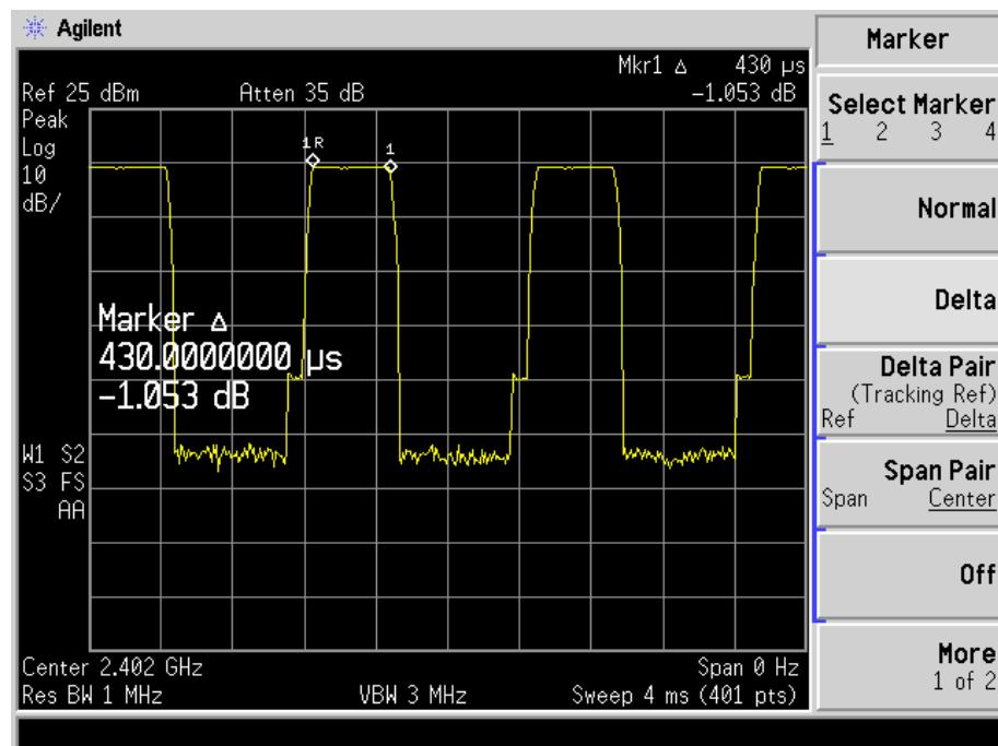
$$\text{DH1 time slot} = 0.43 \text{ (ms)} * (1600/(79)) * 31.6 = 275.2 \text{ (ms)} < 400 \text{ (ms)}$$
