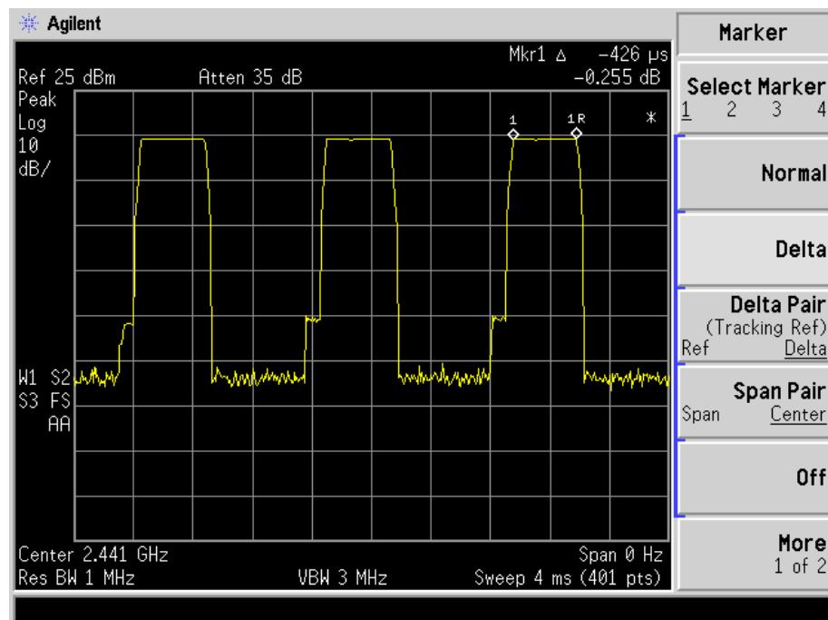
$$\text{DH1 time slot} = 0.426(\text{ms}) * (1600/(79)) * 31.6 = 272.64(\text{ms}) < 400 (\text{ms})$$
